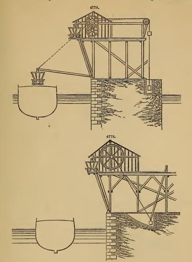
him in 1813, have been generally followed, with various modifications. The principle of all these drops is, that the loaded wagon in its descent raises a counterbalance weight; and when the coals
